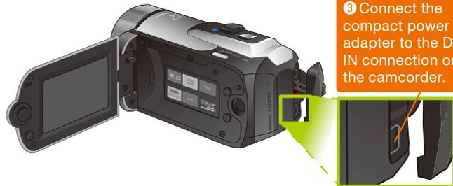
③ Connect the compact power adapter to the DC IN connection on the camcorder.
