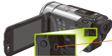
③ Connect the compact power adapter to the DC IN connection on the camcorder.
