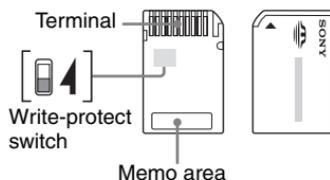
Some “Memory Stick Duo” cards do not have a write-protect switch. On “Memory Stick Duo” with this switch, the position and shape may vary depending on the “Memory Stick Duo”.
