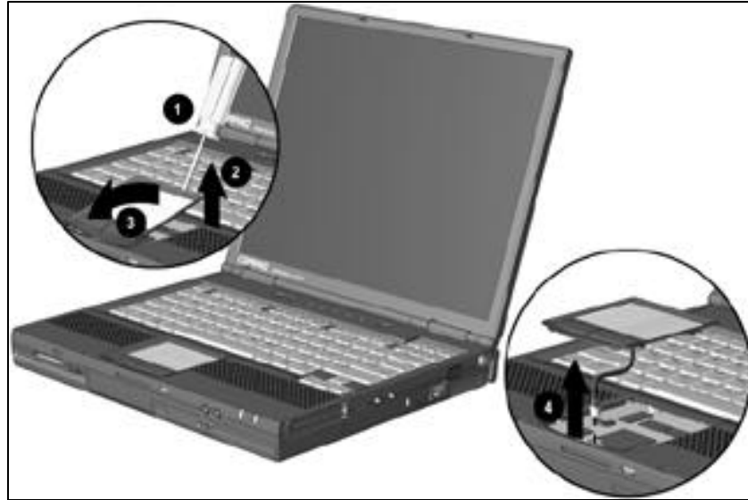
Figure 5-6. Removing the Touch Button
