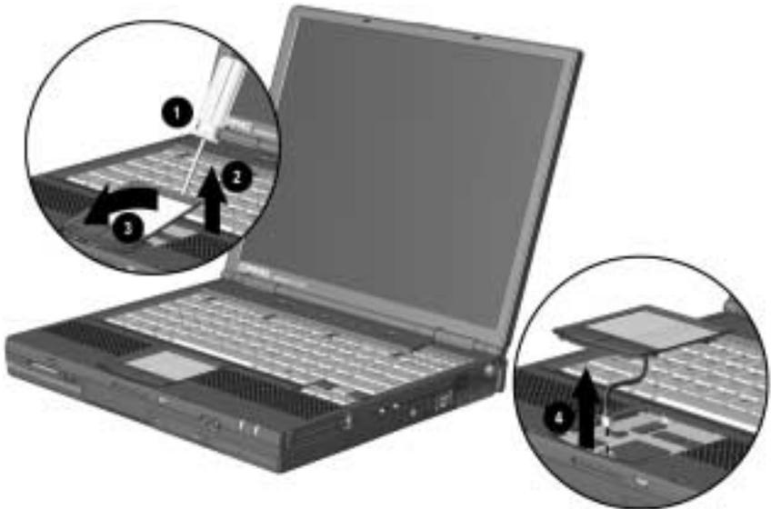
**Figure 5-5.** Removing the Touch Button
