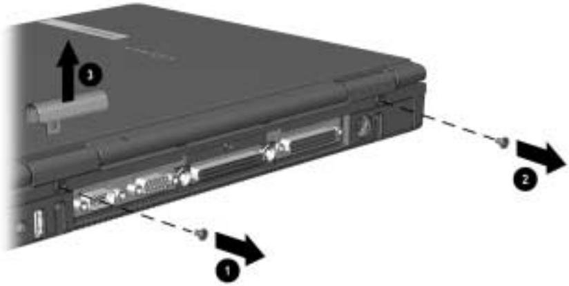
**Figure 5-12.** Removing the Switch and Hinge Cover Screws
