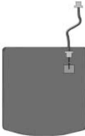
**Figure 5-6.** *Disconnecting the Touch Button Cable*
