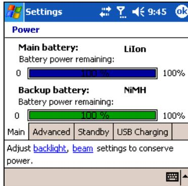
The main battery provides the HP iPAQ with power when it is not physically connected to the cradle or AC adapter. The internal backup battery provides the HP iPAQ with enough power to maintain data when you remove the battery for short periods of time. When the backup battery is fully charged, it maintains data for up to 15 minutes. However, you should always replace the main battery (extended or standard) immediately to minimize the drain on the backup battery.
