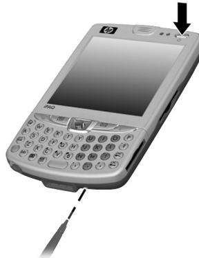
3. Once the HP iPAQ screen fades, release the **Power** button and remove the stylus from the **Reset** button.
