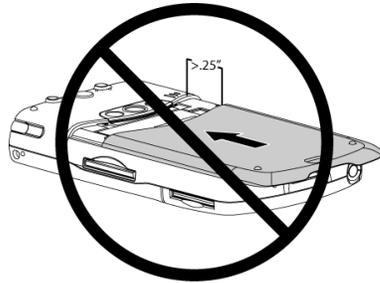
Do not attempt to insert the top two tabs into the unit and then press down the battery cover. This will bend and/or break the hooks on your battery cover.
