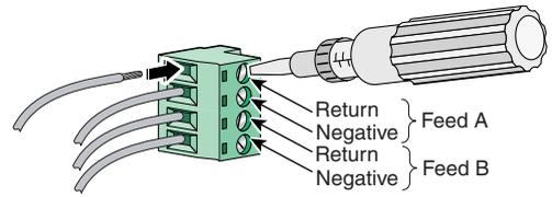
**Step 5** Insert the terminal block plug in the terminal block header on the rear panel of the Catalyst 2950G-24-EI-DC switch or on the front panel of the Catalyst 2950ST-24 LRE 997 switch.
