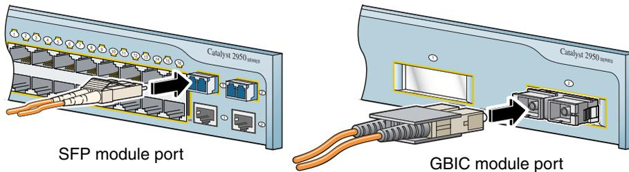
For a list of supported modules, refer to the release notes on Cisco.com. For detailed instructions on installing and removing modules, refer to the documentation that came with the SFP or GBIC module.
