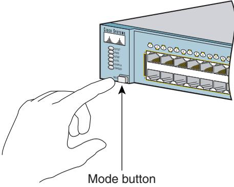
The diagram shows a side view of a network switch. On the left side, there is a control panel with several LEDs labeled SYST, STAT, and RPS. Below these LEDs is a small rectangular button labeled 'Mode button'. A hand is shown with the index finger pointing directly at this button. An arrow points from the text 'Mode button' below the diagram to the button itself. To the right of the control panel is a port block with several RJ45 ports, each with a small LED above it.
