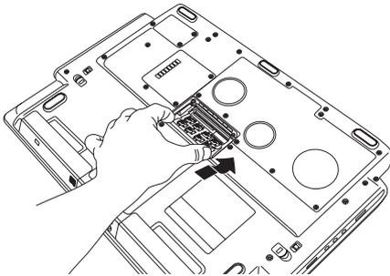
*Inserting the memory module*
