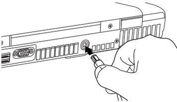
*Sample connecting the AC adapter to the computer*
