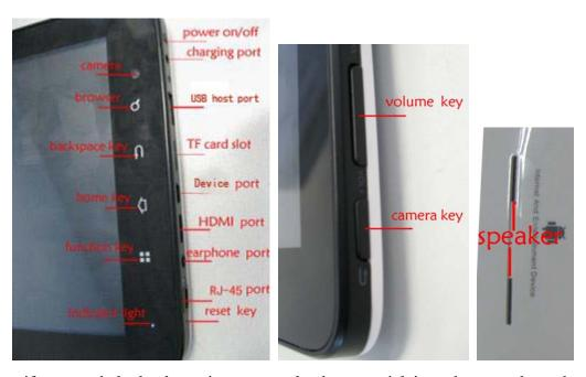
Note: if system halted, please insert one slender material into the reset key ,then system will shutdown.
